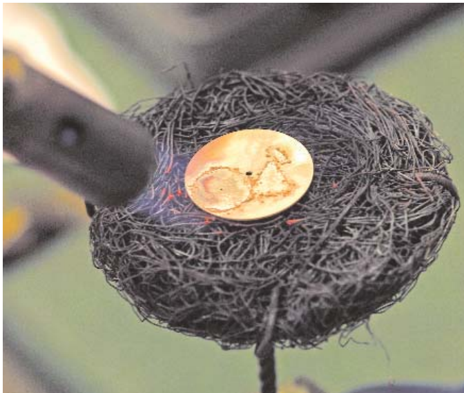
After engine-turning the solid silver parts of the dial are assembled by hard soldering.
