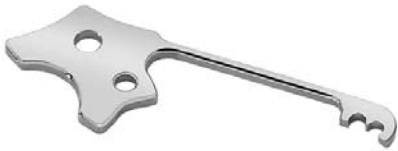
The high-grade setting lever spring, like all other flat steel work in the GREAT Watch, is at least 0.5mm thick, and is black polished & bevelled.
