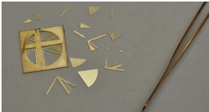
Sterling silver blanks destined to become the watch dial, during their three-month journey of engine-turning, cutting, and soldering.
